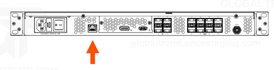
Connect to the processor via the system control LAN. This can be done directly with a laptop or for larger systems, with a wireless router.
