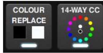
Figure 10-13. ChromaTune pipeline tiles, colour replace and 14 way colour correction
