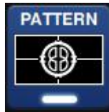
Figure 11-3. Test Pattern pipeline tile, indicating the current active test pattern
